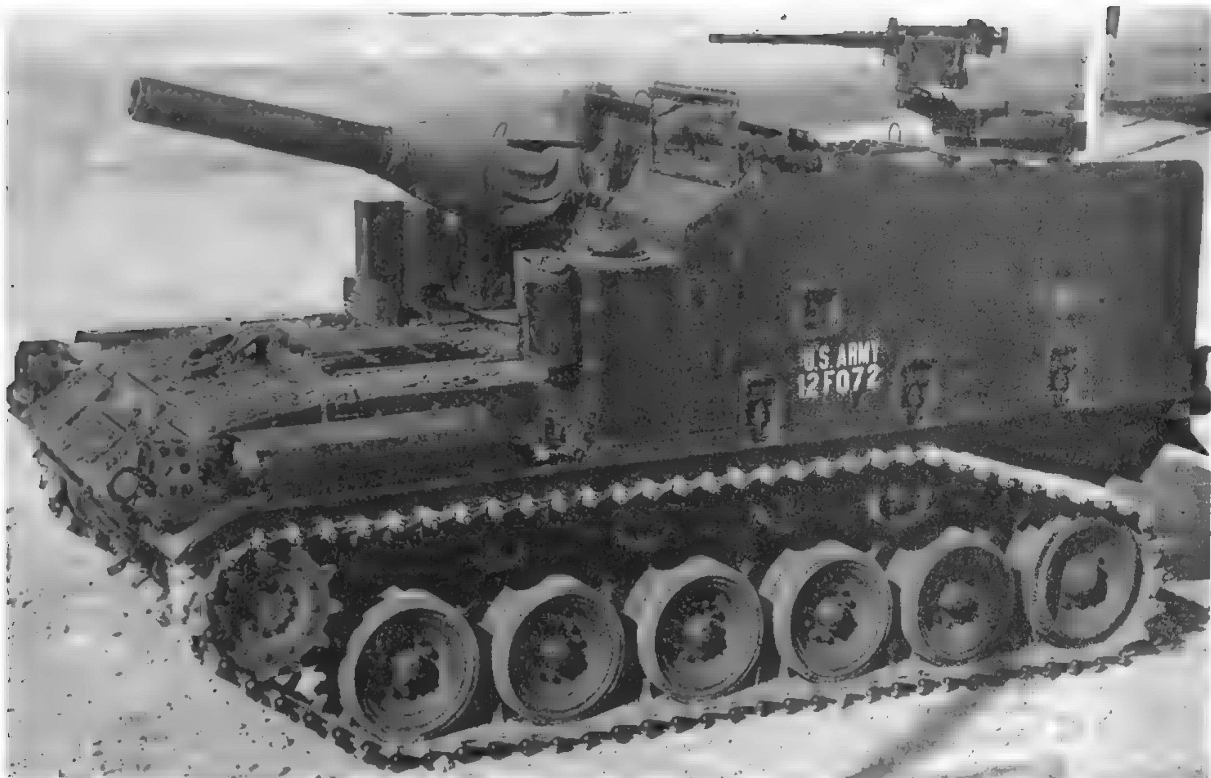
The M44 had an open-topped fighting compartment. It also had a removable windshield and .50-caliber machine gun. (Photo courtesy of the Patton Museum)
